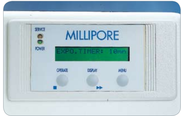
Automatic Sanitization Module control panel
